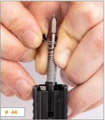
While continuing to hold the firing pin spring down, install the spring cups by placing them on either side of the round part of the firing pin so that they form a circle with the wide part at the top, and then release your grip on the firing pin spring allowing it to move upward and hold the spring cups in place. (# 44)
