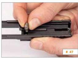
Please ensure the firing pin safety is oriented as shown with the straight side parallel with the slide and the oval/rounded side next to the stripper/feed rail. (# 48/49)
